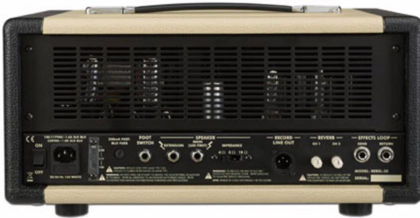
*Fig. 1: Rear-panel options include Silent Speaker mode, which allows you to practice or record without angering the neighbors.*
